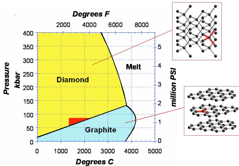
Figure 1 Carbon Phase Diagram
