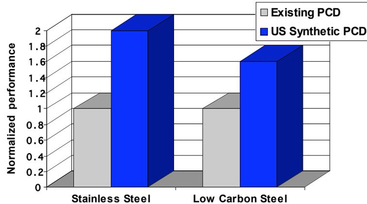
Figure 6 Field test results of US Synthetic PCD Dies
