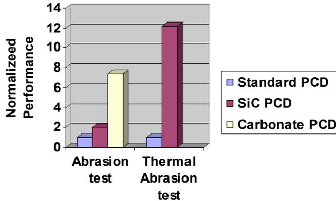
**Figure 7 Abrasion Comparison for SiC and Carbonate PCD**
